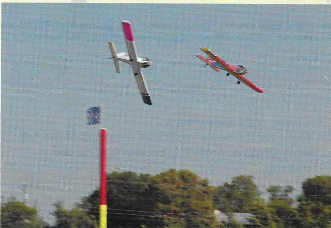
The pylon is typically made from PVC pipe. As shown, the pole is considerably covered with Ethafoam padding (pool noodles).
